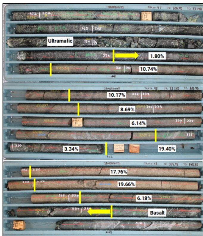
Figure 4: 23MERC112 displaying individual Ni assay results from disseminated to massive sulphide mineralisation
