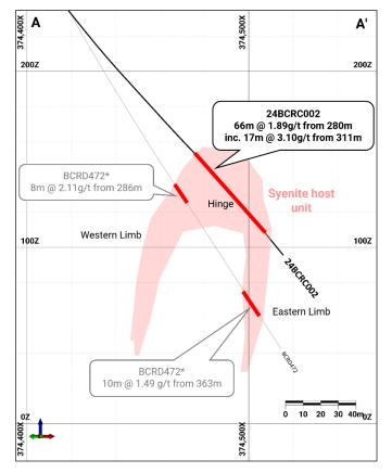
Figure 2 - 24BCRC002 drill section (\*denotes historic drillhole)
