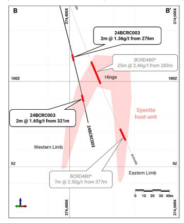
Figure 3 - 24BCRC003 drill section (\* denotes historic drillhole)
