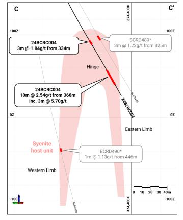
Figure 4 - 24BCRC004 drill section (\*denotes historic drillhole)
