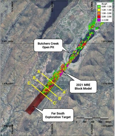
Figure 1 - Plan view of Butchers Creek with related drill section lines
