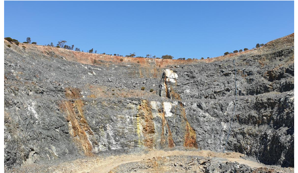
Residual nickel sulphide mineralisation in the southern wall of the 132N Open Pit.
