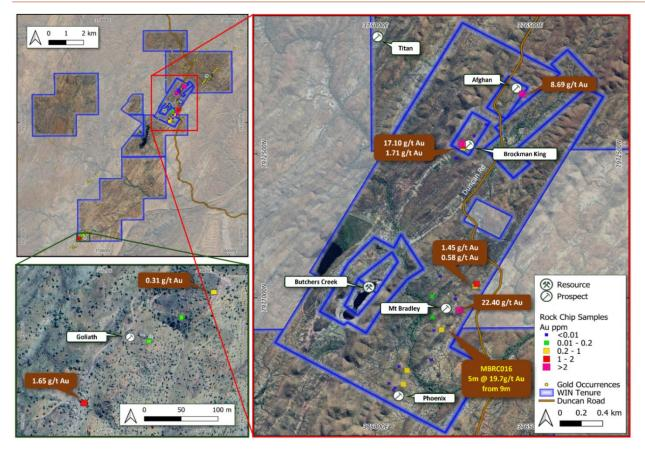
Figure 10 - Rock chip locations showing gold results. High grade rock chip 22.4g/t Au is 230m north of drill hole MBRC016 (5m @ 19.7g/t Au).
