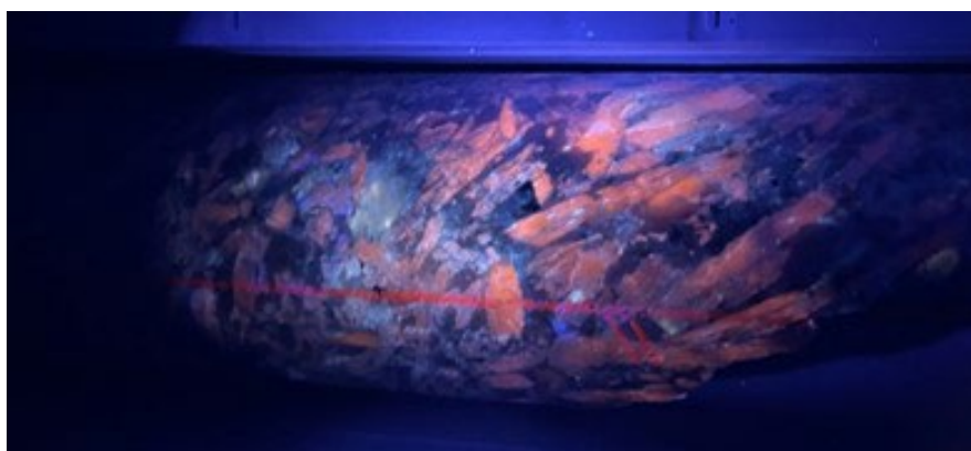
Image 1 - Faraday drill core under UV light, Red/Orange – Spodumene (Lithium bearing mineral \text{LiAlSi}_2\text{O}_6 )
