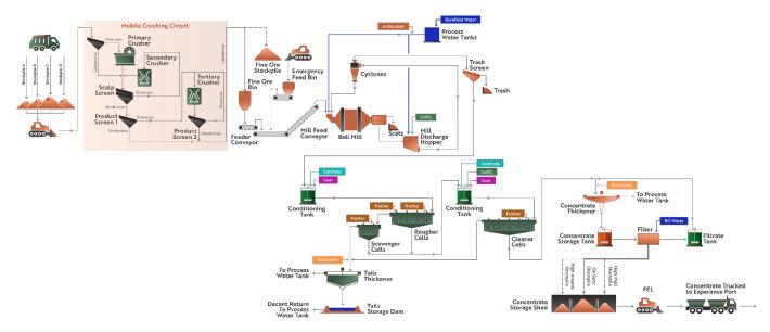
Figure 5: Mt Edwards Nickel Concentrator Flowsheet Schematic
